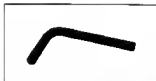
FIGURE A6. PIVOT PIN DETENT INSTALLATION TOOL (P/N 62695) (SEE FIG. 6-3A, PAGE 40 and 6-3B, PAGE 41)
